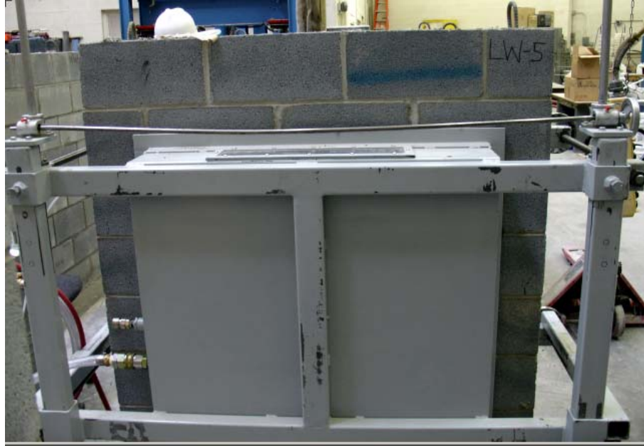
Figure 2: Vacuum cabinet attached to wall assembly
