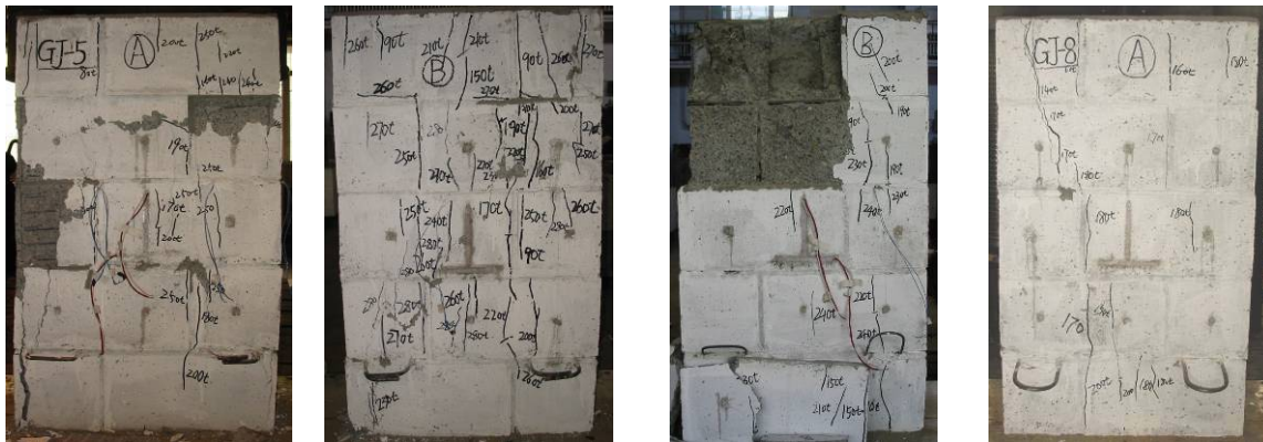
Figure 4: Failure Form of Specimens a) Rectangular hooped bars b) Circular hooped bars c) Rectangular hooped bars inside horizontal joint d) Without hooped bars
