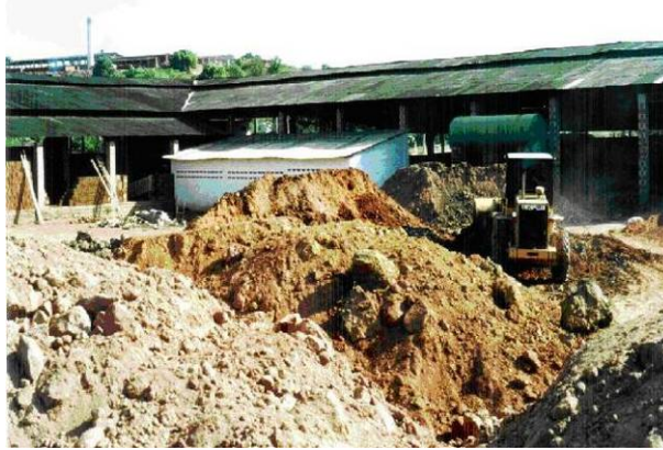
Figure 2: Preparation of the mixture for the ceramic blocks manufacturing
