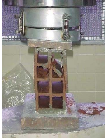
Figure 6: Rupture of the ceramic block
