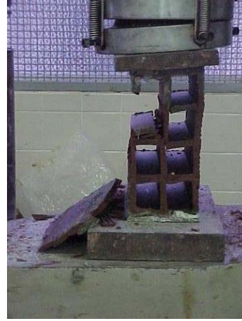
Figure 7: Rupture of the ceramic block
