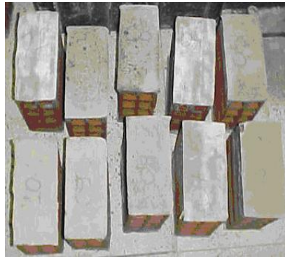
Figura 4: Ceramic blocks capped at both ends
