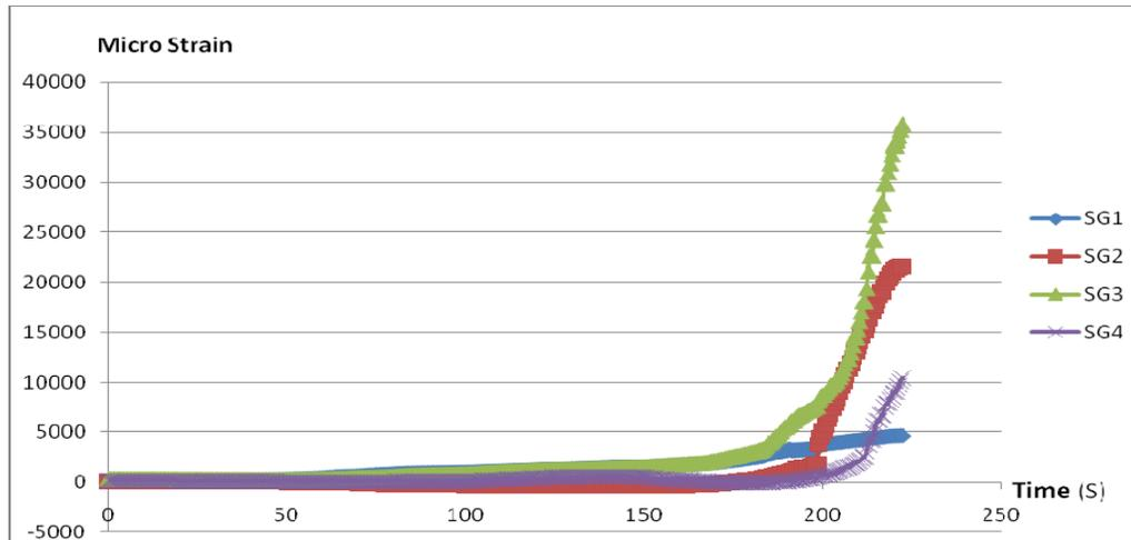
**Figure 6: Typical graph for strain gauge readings in a masonry wall during a test**
