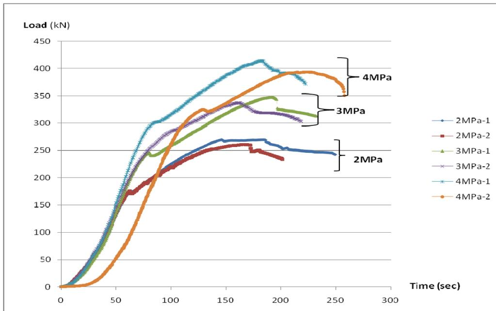
**Figure 7: Typical Lateral Load –Time Curves for different axial stress levels. These are for walls with bed joint reinforcement of diameter 3.7 mm.**
