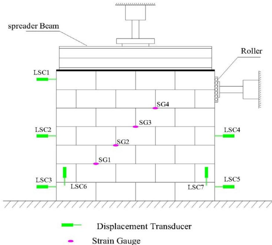
**Figure 4: Distribution of Strain Gauges and Displacement Transducers.**
