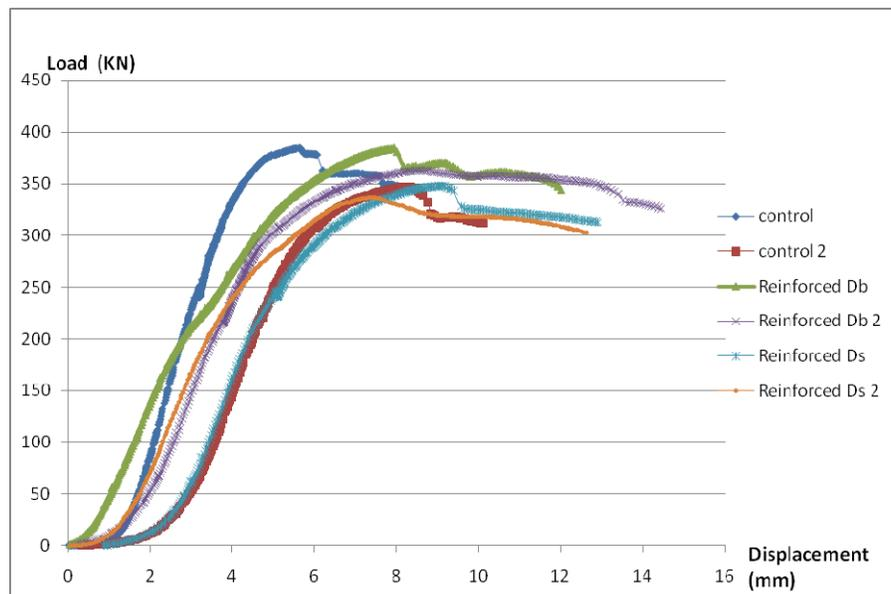
**Figure 5: Typical Lateral Load –Displacement Curves for different types of walls. These are for an axial stress of 3 MPa.**
