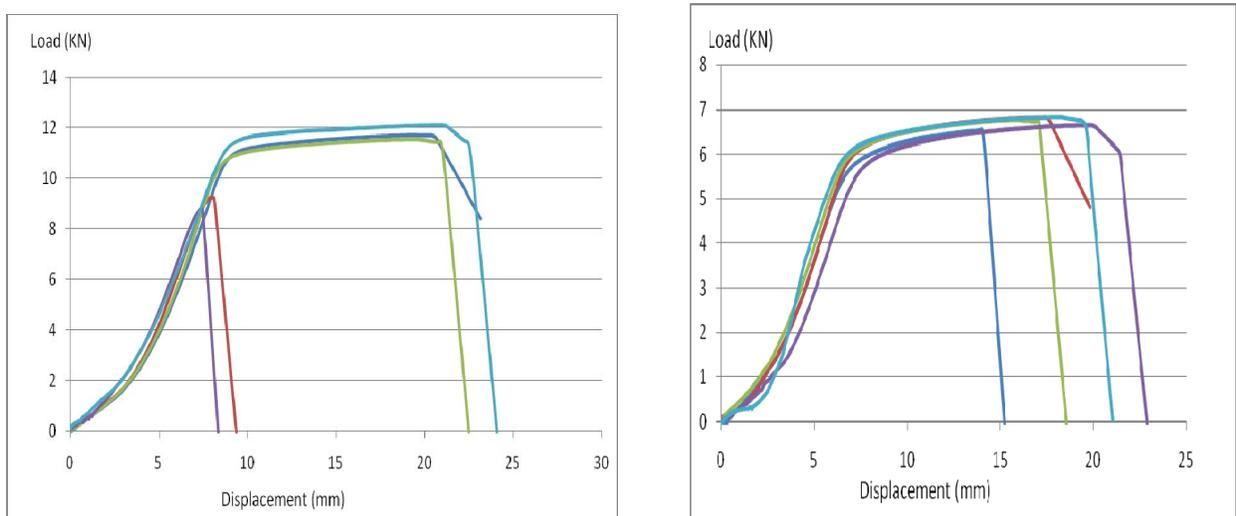
**Figure 1: Load-Displacement curves for the ladder reinforcement used: a) D=4.9 mm and b) D=3.7 mm.**
