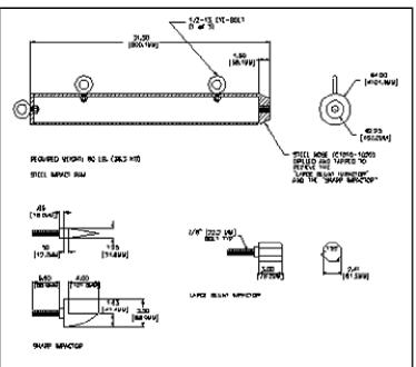
Figure 1 - Pendulum Testing Ram Apparatus
