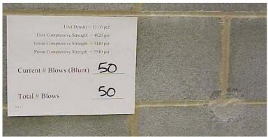
Figure 5 – Test Wall Assembly after 50 Blows
