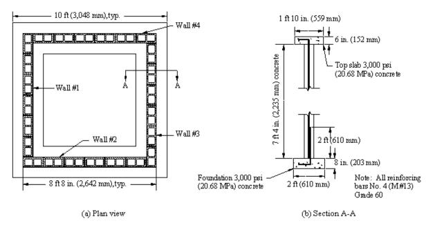
**Figure 2 - Details of Prison Wall Test Panels**
