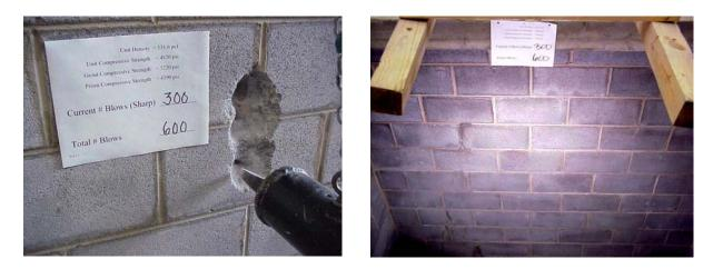
Figure 6 – Typical Wall Condition After 600 Blows – Front Side
