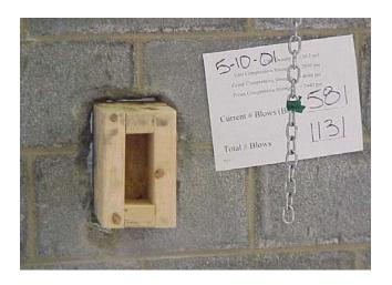
**Figure 8 - Typical Breach Failure**
