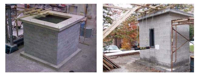
**Figure 3 – Prison Impact Test Walls**
