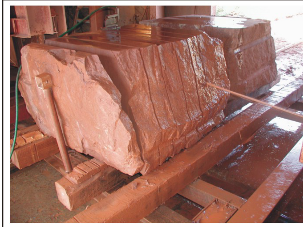
Figure 20 - Cutting quarried stone into slabs prior to shaping and rock face dressing.
