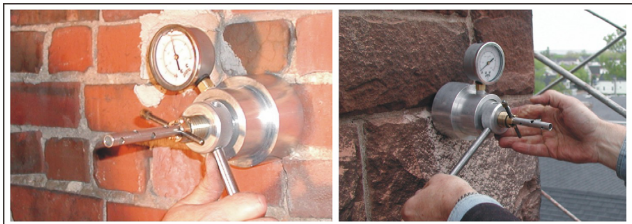
Figure 10 - Tensile strength testing of the masonry ties
