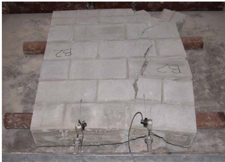
Figure 6 – Typical Cracking in Specimen Set B
