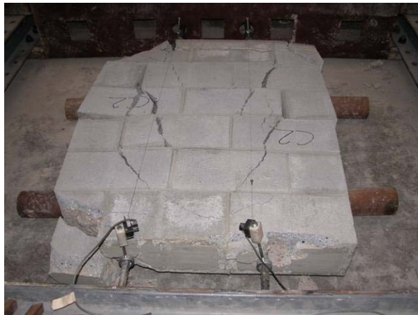
Figure 7 – Typical Cracking in Specimen Set C
