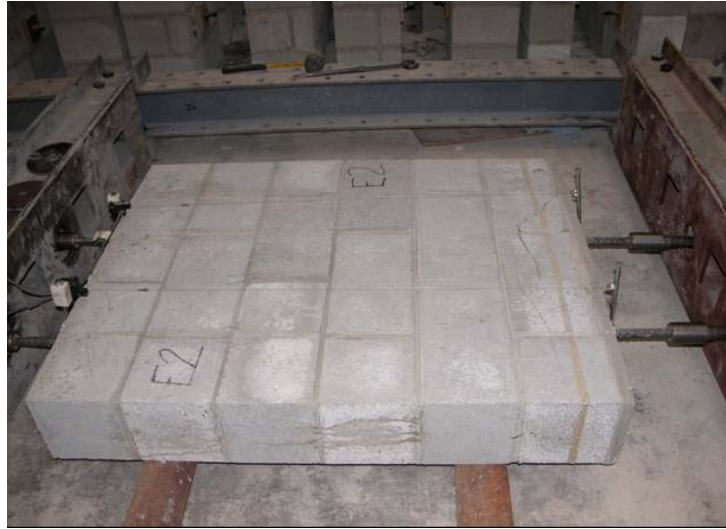
Figure 9 – Typical Cracking in Specimen Set E
