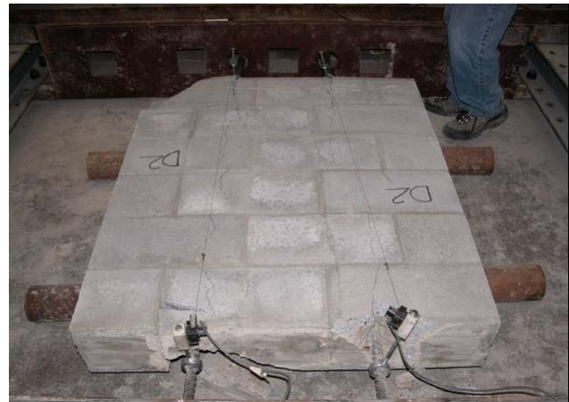
Figure 8 – Typical Cracking in Specimen Set D
