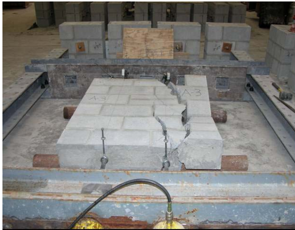
Figure 4 – Typical Cracking in Specimen Set A
