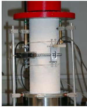
Figure 2 – Compression tests on autoclaved aerated concrete cylinders
