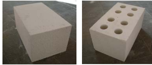
Figure 1 – The masonry units used (length · width · height = 499 · 300 · 249 mm 3 )
