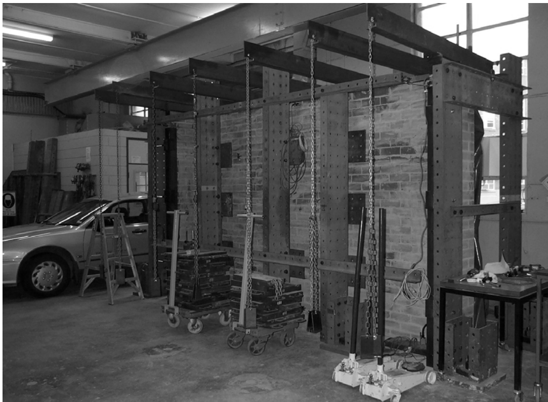
Figure 4 – Overview of Wall Test Set-up
