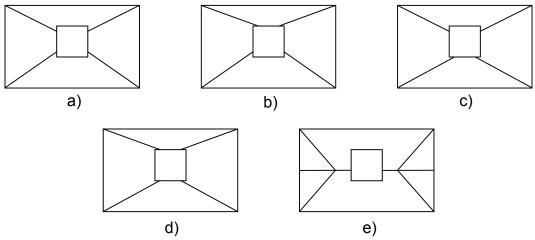
Figure 4 - Potential Collapse Mechanisms for the Failure Line Method
