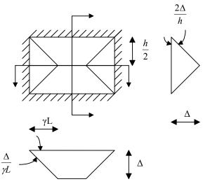
Figure 2 - Relationship between Deflections and Rotations for Failure Line Mechanisms
