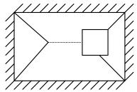
Figure 5 - Critical Failure Line Pattern for Off-Centre Small Window
