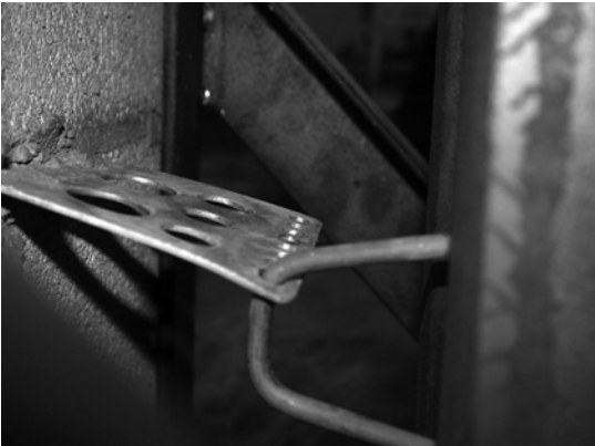
(b) T3 tie after testing (rigid insulation removed for clarity)
