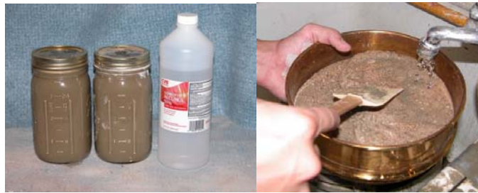
Figure 7 – Mortar Aggregate Ratio Test Samples and Wet Sieving
